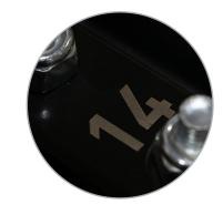
**NOTE** *The blade is marked with a number to signify the corresponding fan size.*
