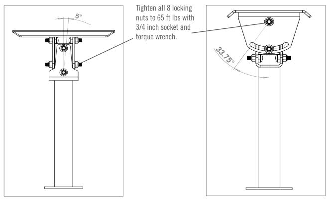
5 degrees of adjustment to accommodate an unlevel beam.
